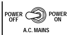
The TIGRIS should be fully powered down and unplugged during severe thunder storms that might cause power failure and line surges, as well as during vacation periods. With the TIGRIS connected to your power source, you should now turn on the A.C. Switch. The front-mounted push button switches should still be in the WARM position.
