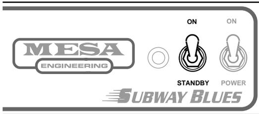
**POWER:** This switch delivers the A.C. POWER to the SUBWAY BLUES. Make sure the unit is grounded (all three terminals of the A.C. POWER cord must be connected whenever possible to avoid injury to the user as well as to the unit) and that the proper voltage is present. Follow the cold start procedure described in the ON / STANDBY section above when powering up your amplifier.
