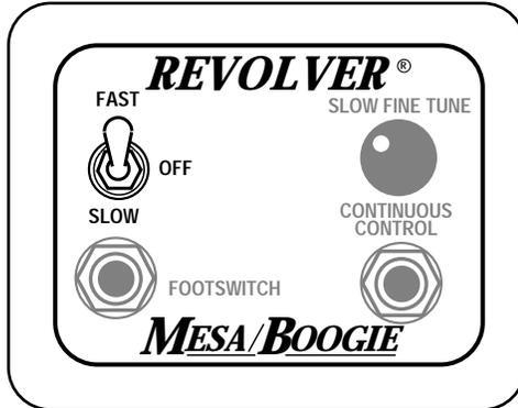
NOTE: The 3 position power switch on the REVOLVER'S Front Panel must be in the SLOW or (down position) for either the Footswitch or the Continuous Control Pedal to function.
