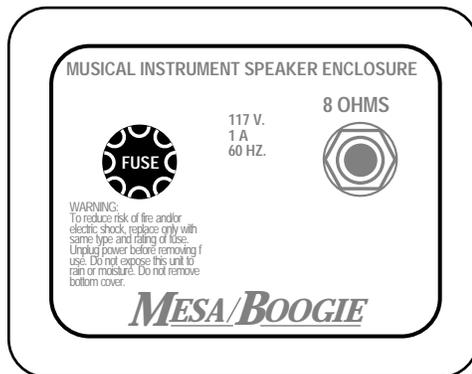
The REVOLVER is protected by two fuses one on the Rear Panel and one inside the cabinet. Should a problem arise, always check both fuses. As always, be sure to disconnect the unit to avoid possible injury and/or causing more damage to the REVOLVER.
