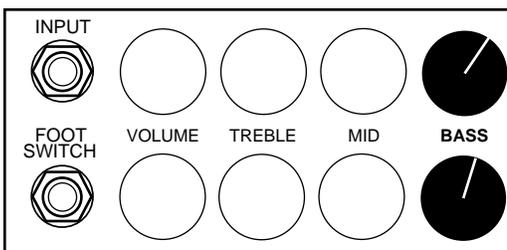
because excessive Bass has been introduced to the pre-amp in the early stages. Try setting the BASS control to 1 for clean sounds in the RHYTHM channel and 2 or below when dialing up high gain overdriven sounds in this channel. In the LEAD channel, try setting the BASS control somewhere between 3 and 4.
