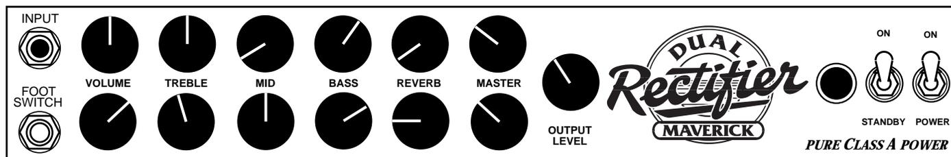
Flip the STANDBY Switch to the ON position and listen to the two channels using either the footswitch or the Channel Select toggle switch found on the Rear Panel. Again, these are merely examples of the two channels. Experimentation leads to finding many different sounds in each channel, and understanding the controls and the way they interact can make this much easier and more fun.
