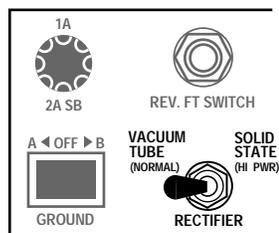
**SOLID STATE (HI POWER)** calls up the silicone diode rectifiers offering more punch, a tighter attack with added brightness and substantially more headroom. This would be the preferred position for loud clean playing or tight rhythmic playing in the Lead channel with a high front end Volume setting (high gain.)
