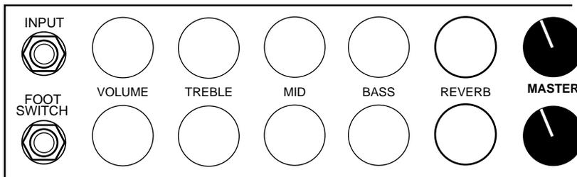
SECOND: They act as effects send controls for each channel in the Effects Loop. As with many of the controls on the MAVERICK, the best results for balance and tone are usually found in the medium range of this control.
