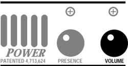
**NOTE:** If only one speaker is to be used on one channel and no speaker load is present on the other, always turn the unused channels VOLUME Control to zero. To prevent oscillation (motorboating like sound) turn the PRESENCE Control of that channel all the way up.
